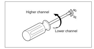
If the TV's channel selector was set to a higher channel than channel 36, turn the RF channel adjustment screw to the right and vice versa.
