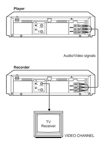
1 Connect the player's AUDIO and VIDEO OUT connectors to the recorder's AUDIO and VIDEO IN connectors.
